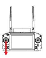
**Option 2.** After landing on the ground, pull the throttle stick down to the lowest position for 3 seconds to stop the propellers
